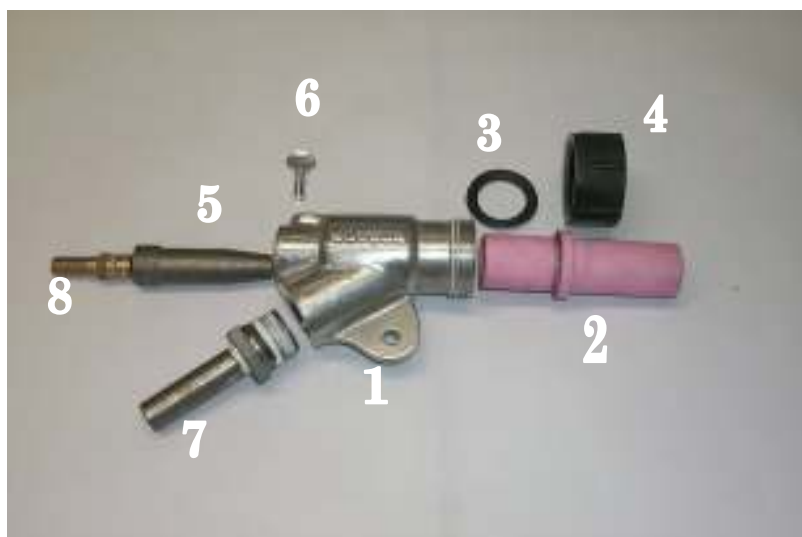
Exploded View of Blast Gun
