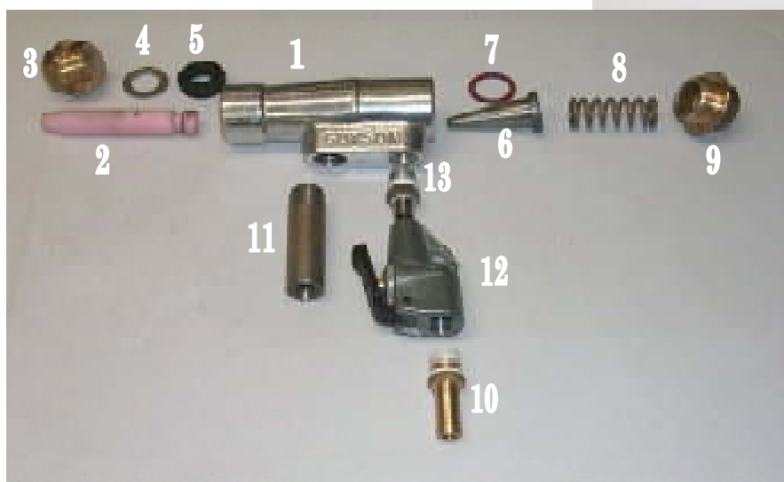
Exploded View of Blast Gun
